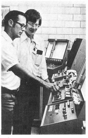
IN THERMAL ANALYSIS LAB Bob Courtney and John Lanoue operate thermogravimetric analysis instruments.
